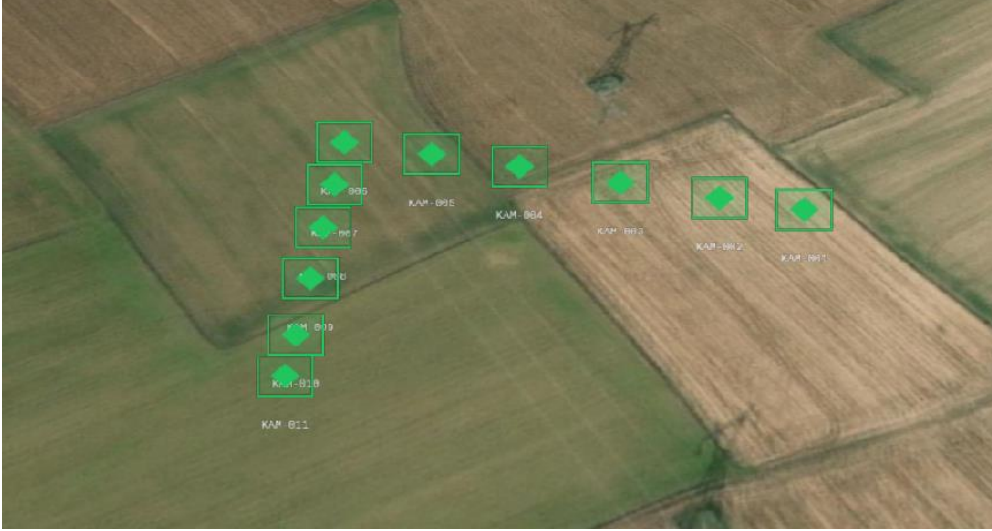
Fig. 5. Cesium-based ground monitoring display showing the eleven-UAV swarm in a V formation.
